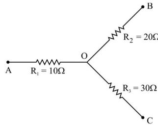
44. Fig. represents a part of closed circuit. The potential difference between A and B i.e.  $V_A - V_B$  is:
